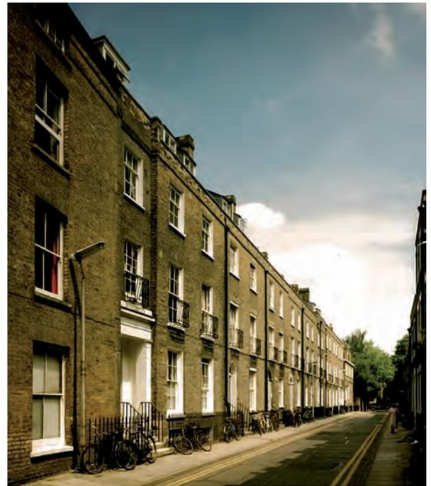
Figure 3: In Georgian streets the small spacing-to-height ratio is compensated for by tall windows. Note how window head height increases for the lower floors which are more heavily obstructed.
