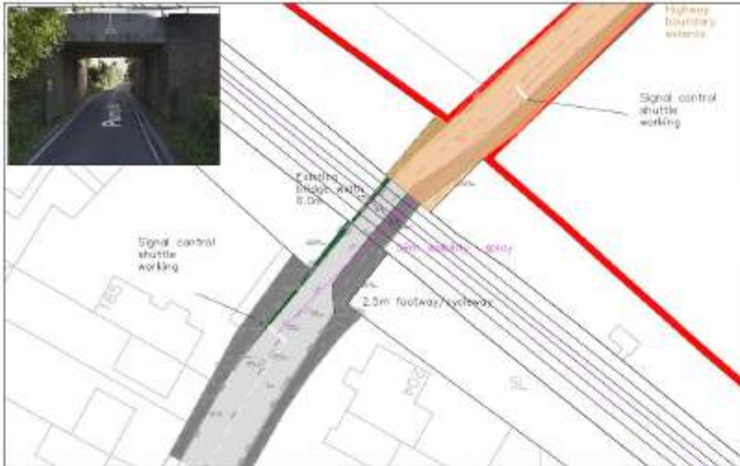
Figure 4 Proposed Pump lane Railway Bridge Improvements
