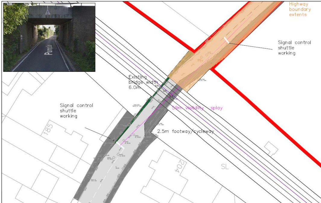
Figure 4 Proposed Pump lane Railway Bridge Improvements
