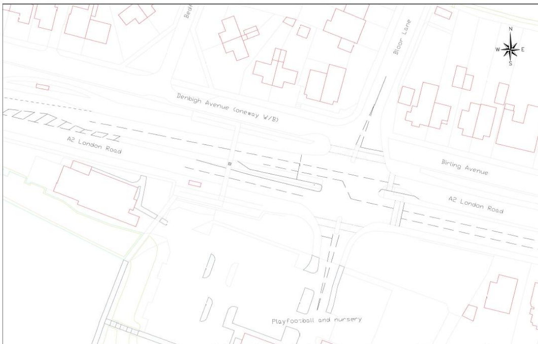
Figure 3 Proposed A2-Bloor Lane Junction Improvement works
