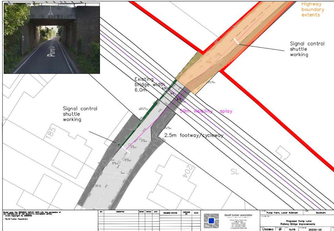
Figure 3 Pump Lane Railway underbridge mitigation
