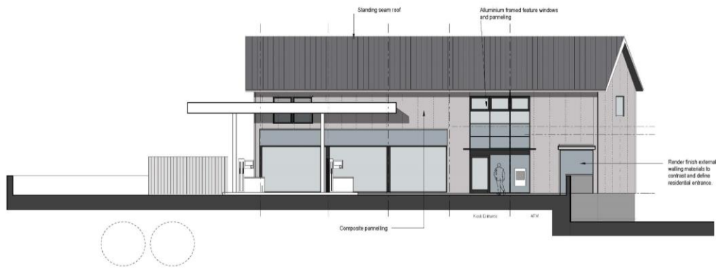
Forecourt Elevation to Drybrook Road
